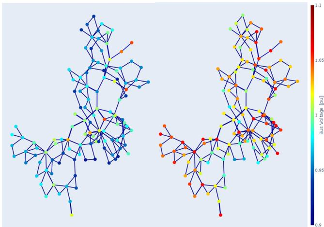
Fig. 4: A visual representation of voltage magnitude in the 118-Bus network at peak demand. Left is shown the DC OPF with AC power flow correction and right is shown the AC OPF.
