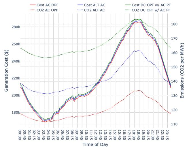
Fig. 3: Generation costs (left) and carbon emissions (right) per 15 minute period over a single day simulation for each of the three dispatch methods considered.
