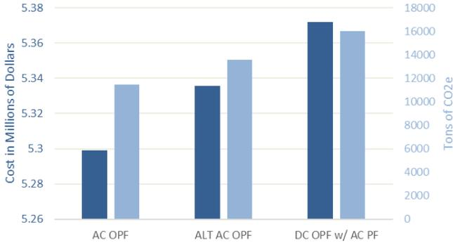
Fig. 1: Generation costs and emissions over a single day simulation for each of the three dispatch methods considered.
