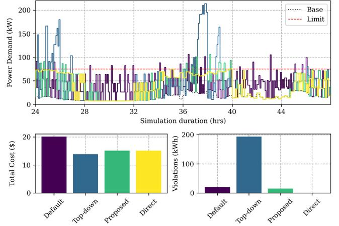
Fig. 7: The results for a case study from 100 homes with smart HVAC systems. Default: the devices act to minimize energy consumption, Top-down: the devices minimize energy cost using LMPs, Proposed: the proposed method where LMPs are altered to protect constraints, Direct: aggregator based control to minimize cost subject to network constraints.
