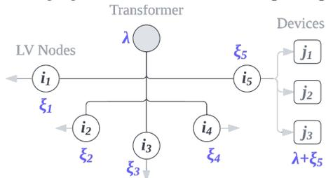
Fig. 2: An example network. Multiple low voltage nodes are connected to a transformer. All devices receive the price  $\lambda$  plus an additional offset  $\xi$  which is specific to their node.
