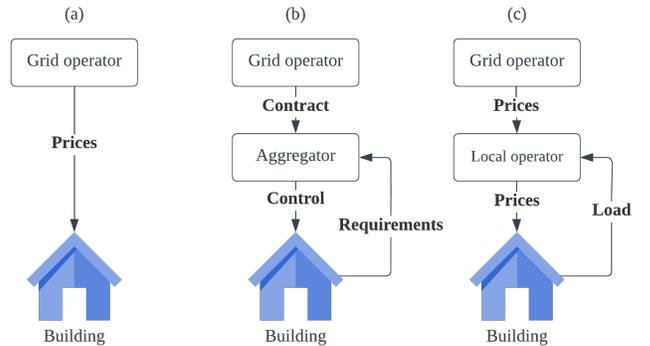
Fig. 1: Three architectures for exploiting distribution level resources for transmission level goals. (a) top-down: where TSO level price signals are passed straight to smart devices, (b) direct control: where a local aggregator takes control of the smart devices, (c) proposed method: where a local operator adjusts the TSO price signals in response to local observations.
