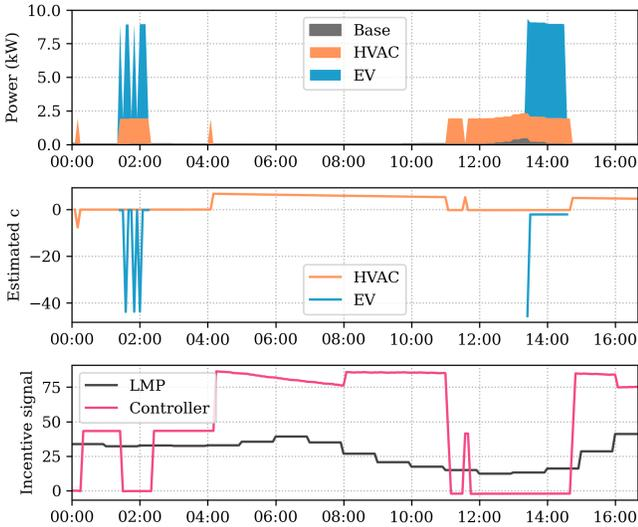
Fig. 8: Illustration of the action of the controller on a single building with both an EV and HVAC. Top: resulting power consumption, middle: controller estimated value of device point, bottom: original and adjusted price signal.
