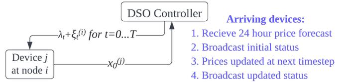
Fig. 3: The communication process when a device is activated.
